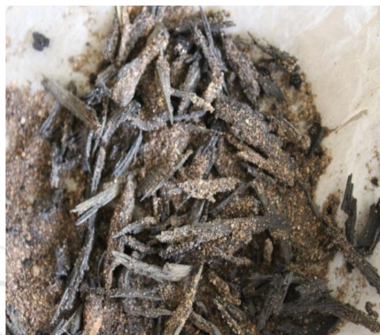
Figure 4: Sand coated tyre chips
