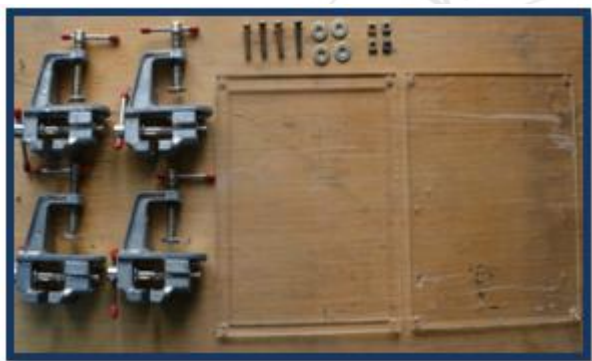
Figure 1: Custom made plastic mold parts.
