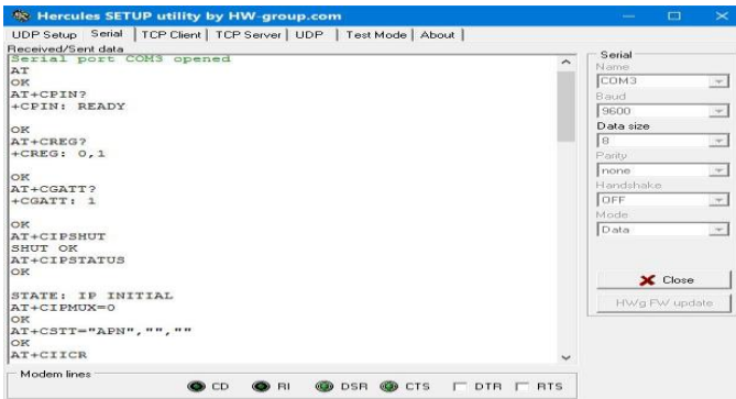
Figure 5: TCP/IP using in SIM800C with Hercules SETUP Utility
