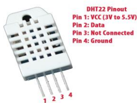
Figure 3: DHT-22 (Temperature Sensor)
