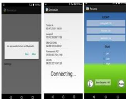
**Figure 5:** GUI of Android Application showing process of connecting to Bluetooth module
