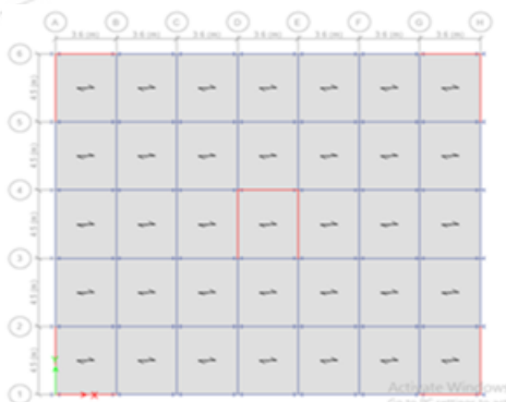
Model 10: SPSW at All Corner Positions and At Core
