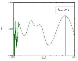
Figure 2: UV Spectrum of Tenoxicam
