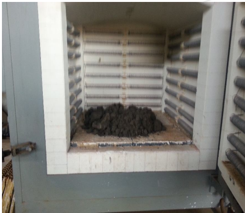
Figure 1: Esklo s.r.o heating kiln (Sample in position)
