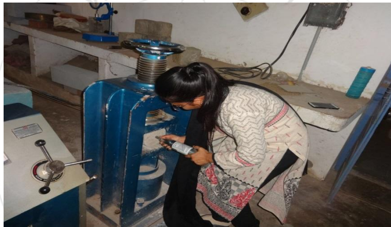
Figure 3: Rebound Hammer Testing in Laboratory
