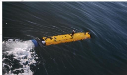
**Figure 5:** AUV to detect mine like objects
