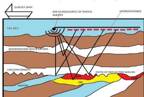
Figure 2: Underwater Seismic Monitoring
