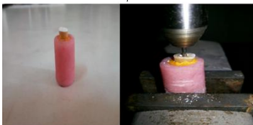
Figure 2: Right, the tested sample preparation, on the left is specimen under load
