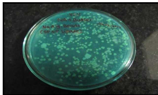
Figure 2: Detection of lipolysis of unsalted butter by Immobilized SP45 Lipase
