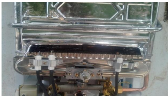
Figure 2: Internal Detail of Gas Geyser Gas Geyser
