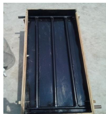
Figure 3: Solar Water Heater
