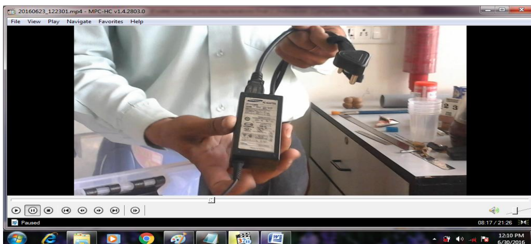
Picture 11c- This is the 19V.3.16A laptop charger/adopter for power supply to device.
