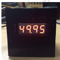
Figure 9: Test and result of line frequency measurement (at the testing stage)
