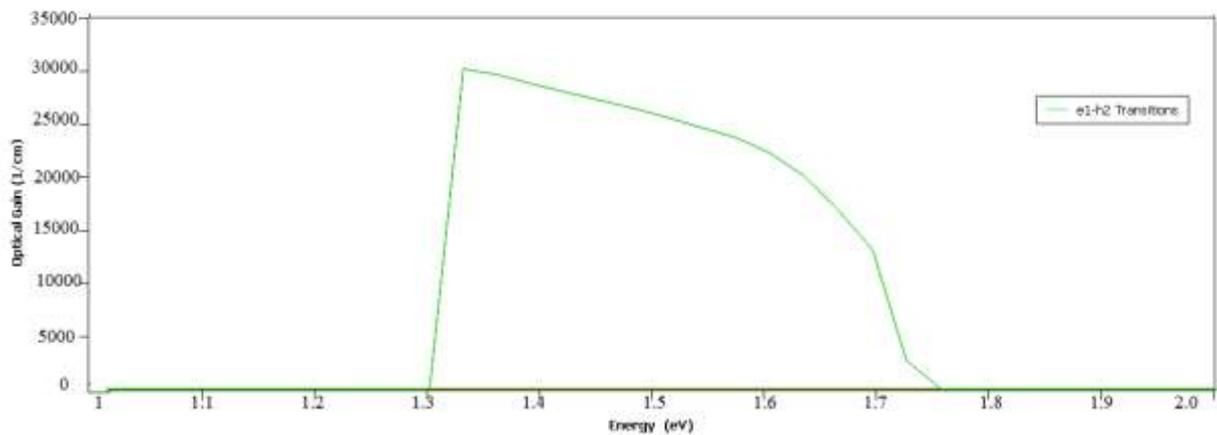
Figure 5: Optical gain as a function of photon energy for Type-I hetrostructure InGaN/GaN at 300K
