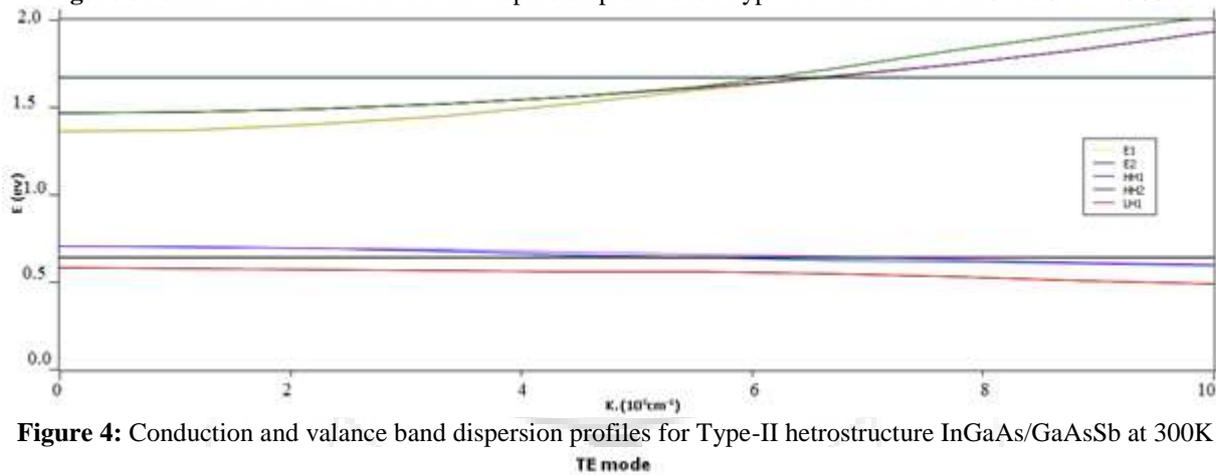
Figure 4: Conduction and valance band dispersion profiles for Type-II hetrostructure InGaAs/GaAsSb at 300K
