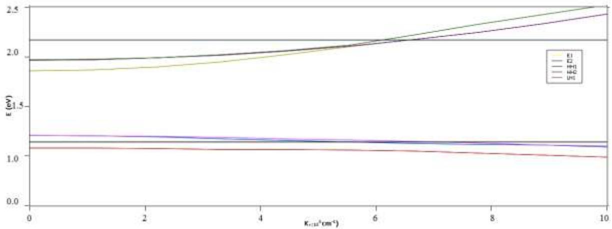
Figure 3: Conduction and valance band dispersion profiles for Type-I hetrostructure InGaN/GaN at 300K
