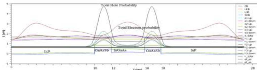
**Figure 2:** Wavefunction waveform for Type-II heterostructure InGaAs/GaAsSb
