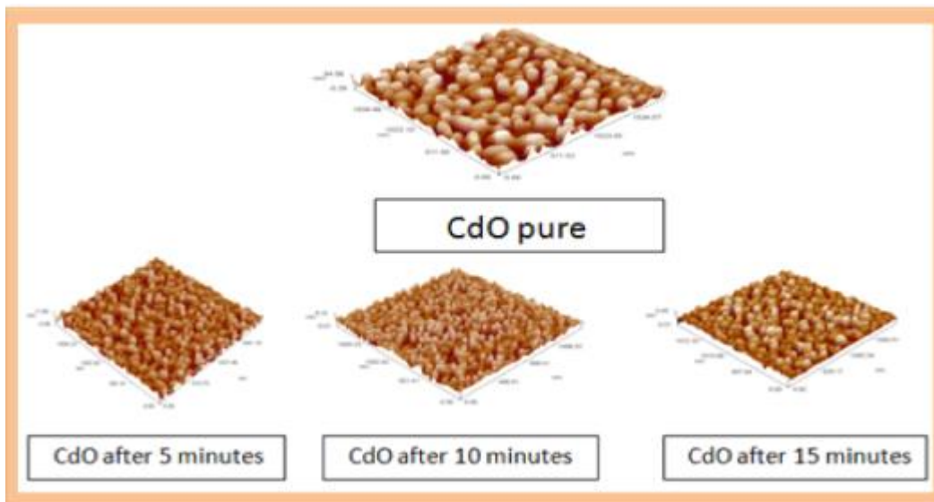
Figure 4: Two-dimensional AFM images of CdO films after and before exposure to non-thermal plasma
