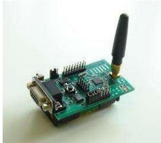
Figure 8: Wireless sensor unit
