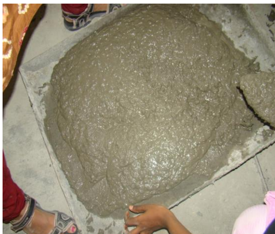
Figure 3: Fresh concrete of SCC
