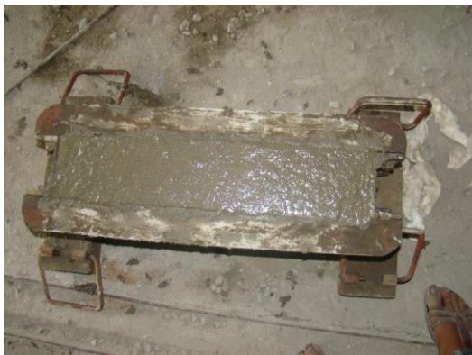
Figure 2: Casting of Prism
