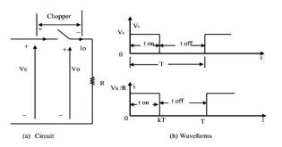
3.1 Chopper circuit diagram and its voltage and current waveform
