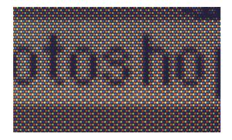
The light and dark tones are created by varying the amount of electricity the electron gun shoots at each pixel. The more electrons the brighter the color. The brightest area around the lettering is what you would see as white when you look at the screen. Because they are too small for our eyes to separate, the red, green and blue lights are seen as white when they reach our brains.
