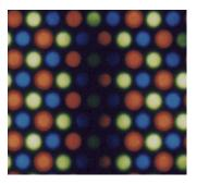
Each of those triangular clusters of a red, green and blue dot is the method your monitor uses to describe each of those pixels we saw above in the can of green beans photo. A square pixel is displayed by a 3-color cluster of phosphor dots on the monitor.
