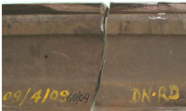
Figure 5: Rail pieces in juxtaposition exhibiting angle of inclination (Approximately 6 degree from vertical) of Transverse Defect. Ultrasonic test report of the rail less than 15 days prior to failure did not indicate any defect. (Courtesy: Ref- 7)
