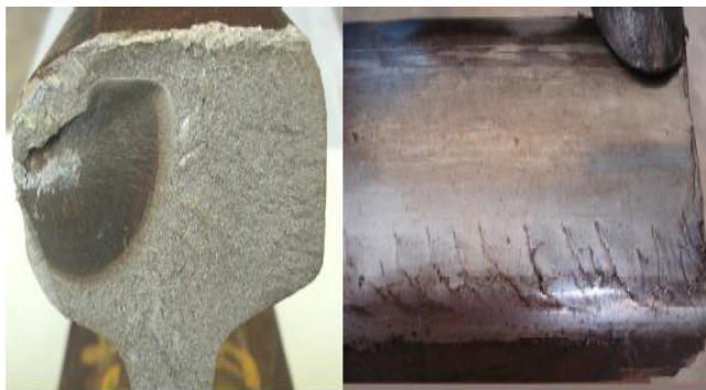
Figure 4: Transverse Defect in UIC 60, 880 Grade Rail covering 30% of railhead area leading to derailment at New Faridabad Station in April 09. Nucleus of fracture initiation corresponds to landing of shear crack present on gauge side of rail table. Adjoining photo shows extent of Head Checks at the location. (Courtesy: Ref- 7)
