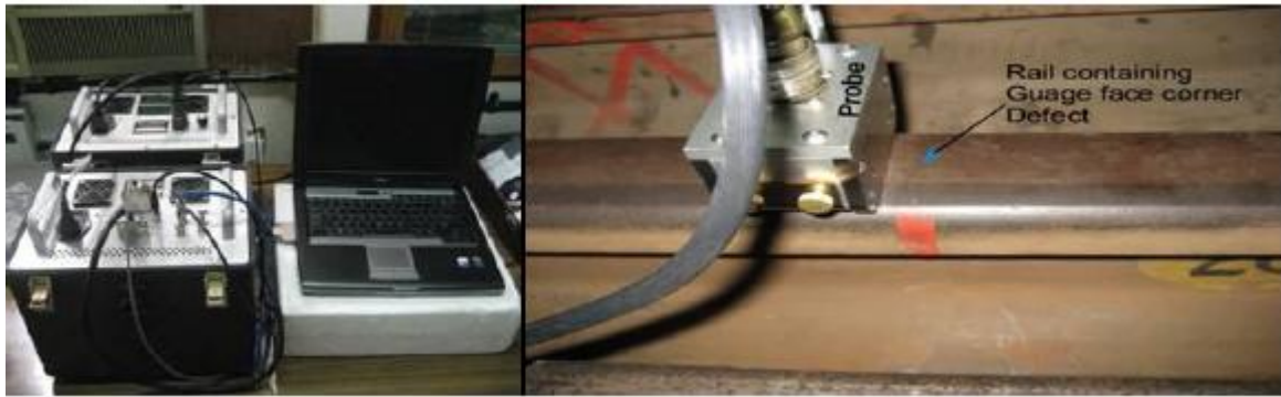
Figure 25: Power Box Set up from Innerspec and Testing of Rail Containing Natural GFC defect (Courtesy: Ref-7)
