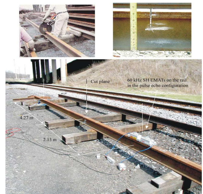
Figure 18: Rail cutting site. Bottom photograph shows the arrangement for the 60 KHz SH EMAT evaluation (Courtesy: Ref-8)
