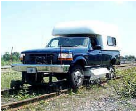
Figure 24: Integrated mobile inspection system. Designed transducer carriage and holder. (Courtesy: A.Chahbaz, M.Brassard and A. Pelletier, Mobile Inspection System for Rail Integrity Assessment. WCNDT 2000)
