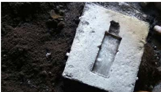
Figure 3: Die which is used to pour the molten material of Al6082 and TiB 2
