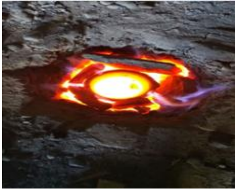
Figure 1: Al 6082 granules were melting in the furnace.
