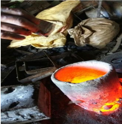
Figure 2: In the melted Al6082 TiB 2 of 15 grams was mixing
