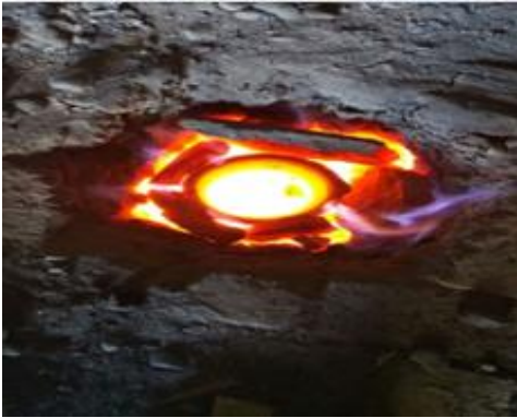
Figure 1: Al 6082 granules were melting in the furnace.
