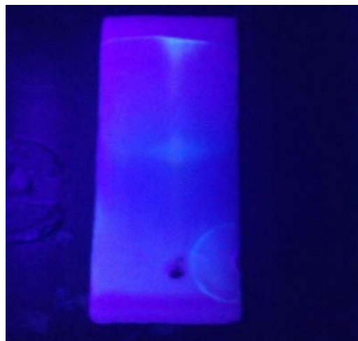
Figure 1: Qualitative analysis by Thin Layer Chromatography of root extract of Dipsicussinermus using Ethyl acetate: methanol(1:1). The R f Value of produced content of root is 1.354.
