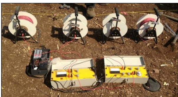
Image 5.1: Photo showing connection for resistivity method
