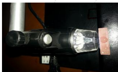
Figure 3: Measuring contact angle by Digital microscope with specimen
