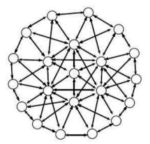
Figure 1: Flooding a Packet in a Wireless Multi-hop Network
