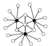
**Multi Point Relay Node Selection:** Multipoint relays plays an important role in minimizing the overhead which is created by redundant retransmissions in the same region by flooding messages in the network. every node selects a set of nodes in its 1 hop neighborhood that are known as multipoint relays (MPR) and they are responsible for retransmission of message in the network. MPR set is selected in such a way that it may coverall the 2-hop nodes i.e. in terms of radio range.
