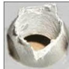
Figure 3: Bush formed after drilling
