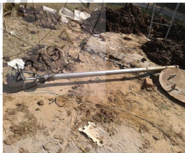
Figure 1: light weight Screw press machine with 1 H.P motor (4inch x 9 feet long)
