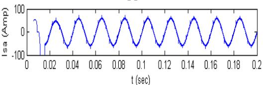
The source current is very much sinusoidal but with spikes. The results obtained for Proportionate (P), Integral (I), PI and PID controllers are as follows:
