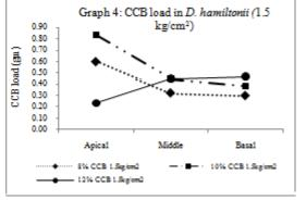
The tests of significance for preservative (CCB) loaded in of *B. pallida* and *D. hamiltonii* was significant among the treatments at 0.05% level of probability (Tables: 3 to 8)
