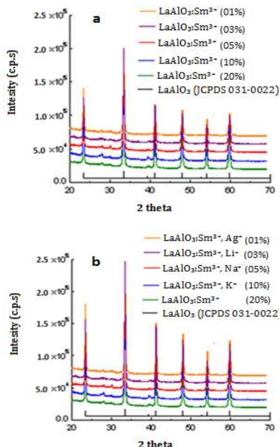
**Figure 1:** XRD spectra of (a)  $\text{LaAlO}_3:\text{Sm}^{3+}$  (b)  $\text{LaAlO}_3:\text{Sm}^{3+}$  [ $\text{Li}^+$ ,  $\text{Na}^+$ ,  $\text{K}^+$ ,  $\text{Ag}^+$ ] phosphors showing sharp xrd peaks.
