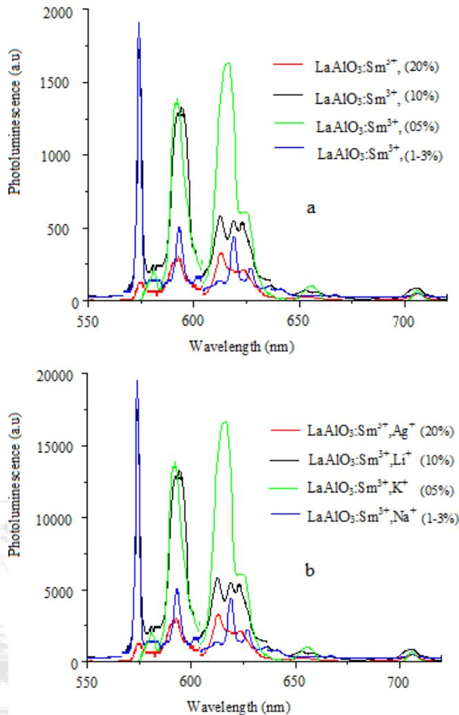
**Figure 3:** PL spectra of (a)  $\text{LaAlO}_3:\text{Sm}^{3+}$  (b)  $\text{LaAlO}_3:\text{Sm}^{3+}$  [ $\text{Li}^+$ ,  $\text{Na}^+$ ,  $\text{K}^+$ ,  $\text{Ag}^+$ ] phosphors showing enhanced yellow, orangish-yellow & orangish-red emission.
