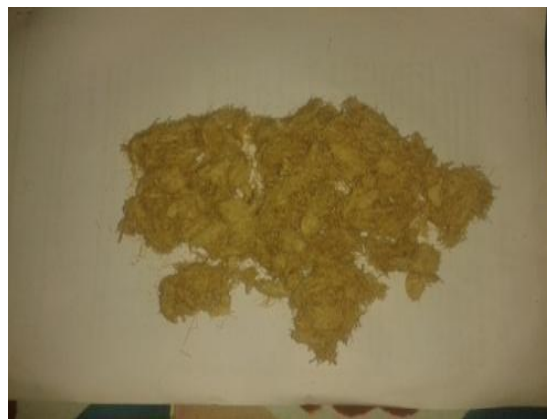
Figure 3.2: Obtained Treated Cellulose from Cross and Bevan method
