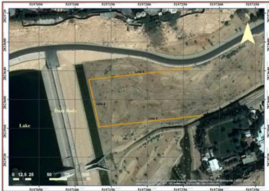
Figure 4: Marked lines representing the GPR traverses next to the dam site.
