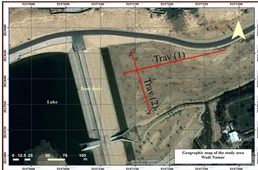
Figure 7: Red lines representing the ERT and Seismic Refraction traverses (Trav (1), (2)); Trav (1) perpendicular and Trav (2) parallel to the dam site.
