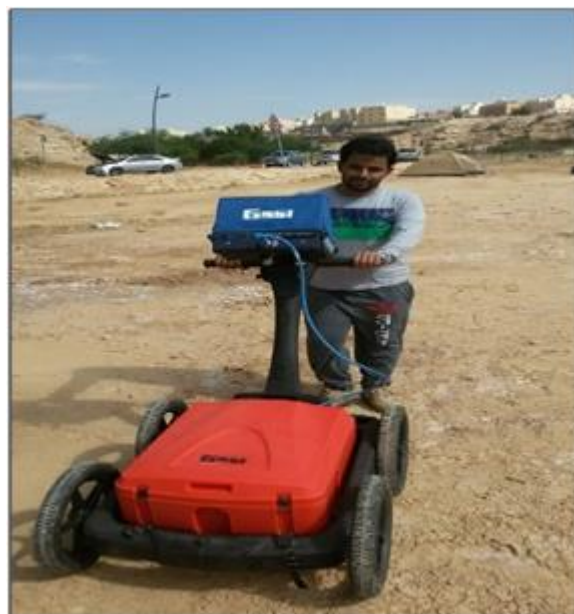
Figure 3: GPR unit used for data acquisition.
