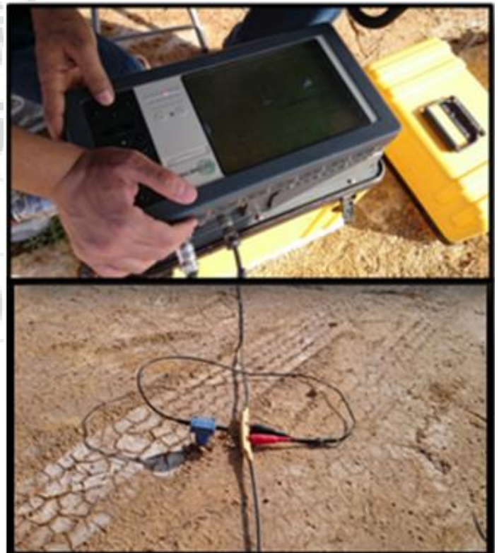
Figure 6: Seismic Refraction Survey
