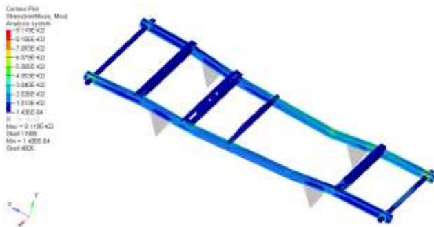
Figure 10: Stress plot for chassis of the vehicle during right cornering
