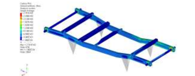
Figure 13: Stress plot for chassis of the vehicle during left cornering
