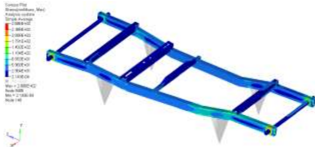
Figure 14: Stress plot for chassis of the vehicle during right cornering
