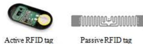
Figure 4(a): Types of RFID tags
