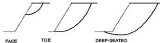
Figure 5: different types of circular failure
