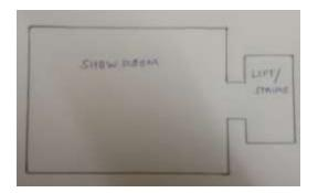
Building consisting of two blocks, Show room (functional block) and Lift / Stairs etc (service block). The service block is structurally independent of functional block.
