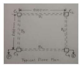
The typical floor plan of G + 4 showroom building is shown above of area 48 Sq.m.
