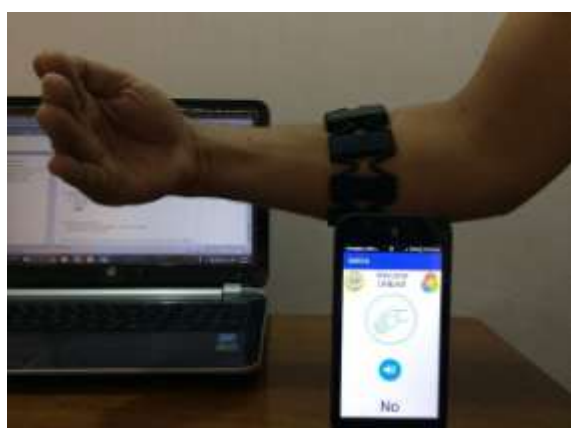
Figure 8: The Gesture “WaveIn” with its Related Word “NO” on the Smartphone Screen
