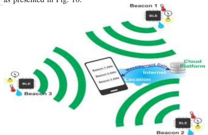
Figure 10: Environmental monitoring system based on BLE.
