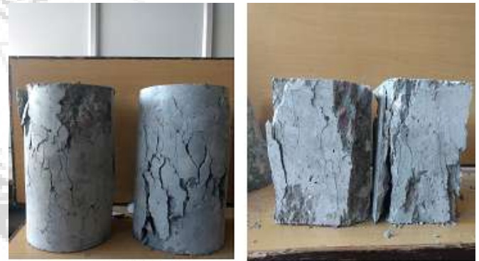
M25 (ACI) M25 (BIS) Figure 5.6: Cracking pattern of M25
