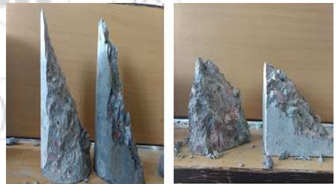
M35 (ACI) M35 (BIS) Figure 5.7: Cracking pattern of M35
