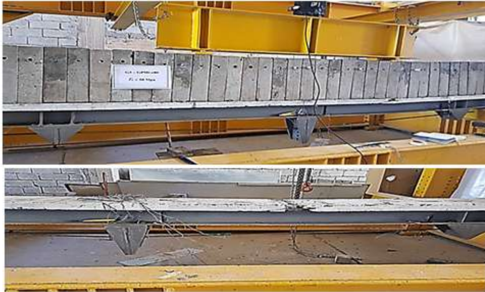
Figure 7: The Mode of Failure of the Steel Girder (GP9D-e160) G2
