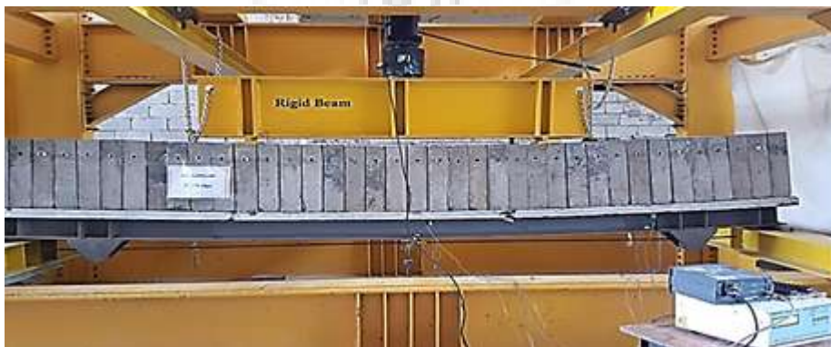
Figure 4: Loading System in the Testing Machine
