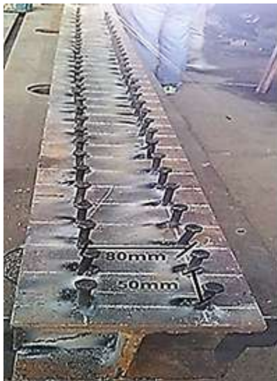
(b) Details and distribution of shear connector for Bridge Model
