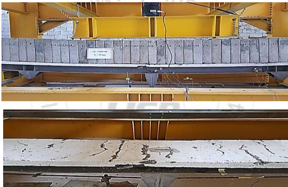
Figure 10: The Mode of Failure of the Steel Girder (GP9D-e160) G4
