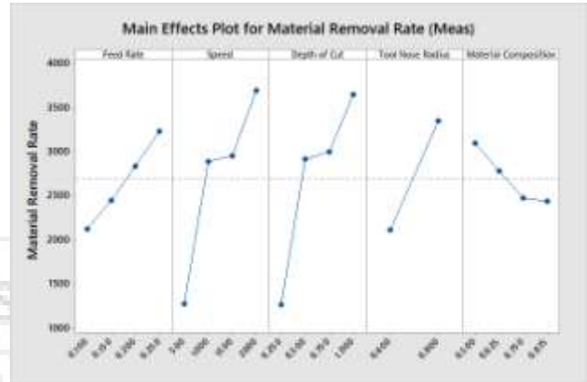
Figure 2: Main effects plot for Material Removal Rate vs cutting parameters
