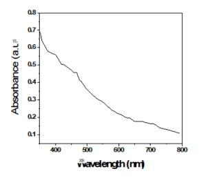
UV-Visible absorption spectrum of MnS nanoparticles
