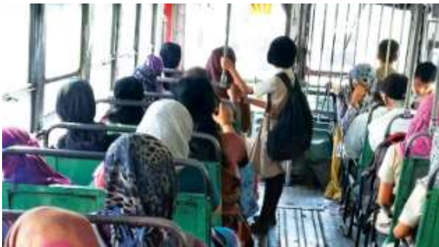
Figure 4: Holding bars are missing
