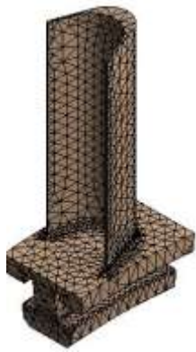
Figure 4: A mathematical model of 70mm blade
