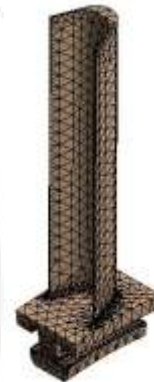
Figure 7: A mathematical model of 120mm blade
