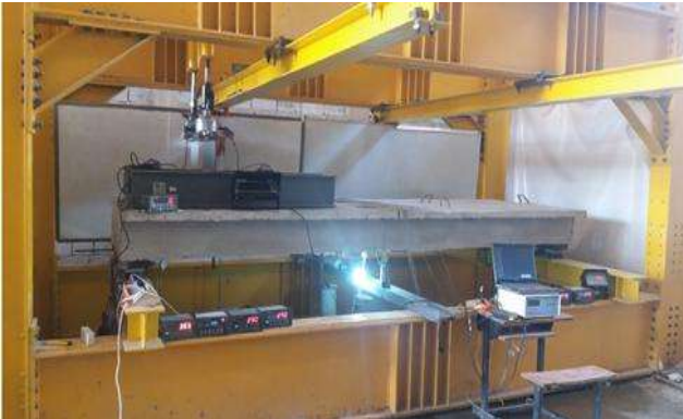
Figure 14: Two design truck at both lane (load case III)
