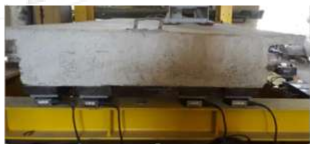
Figure 7: Load cell position under bridge girder left side
