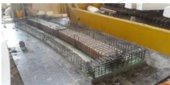
Figure 3: First stage of model construction (Model BGC R 12.5)
