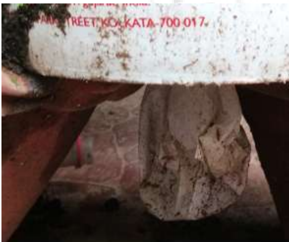
Figure 2.17: Leachate collected after 15 days
