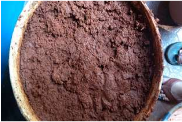
Figure 2.15: Compacted layer of red soil -12% bentonite on garbage
