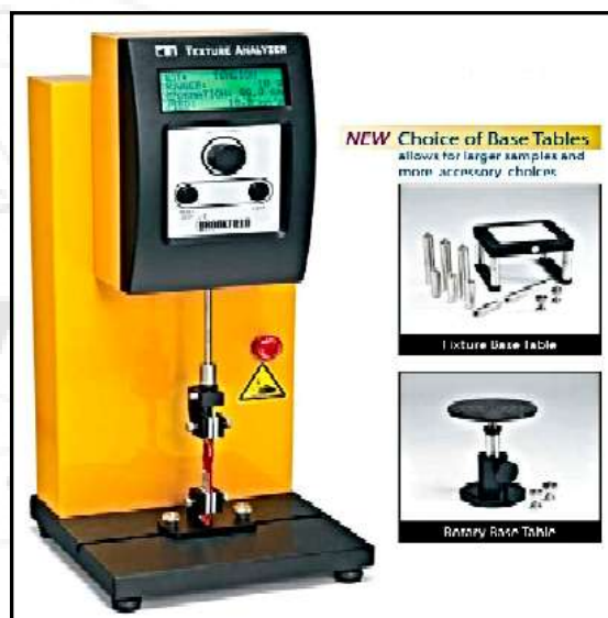
Figure1: Image of CT3 texture analyser used for measurement of mechanical properties.
