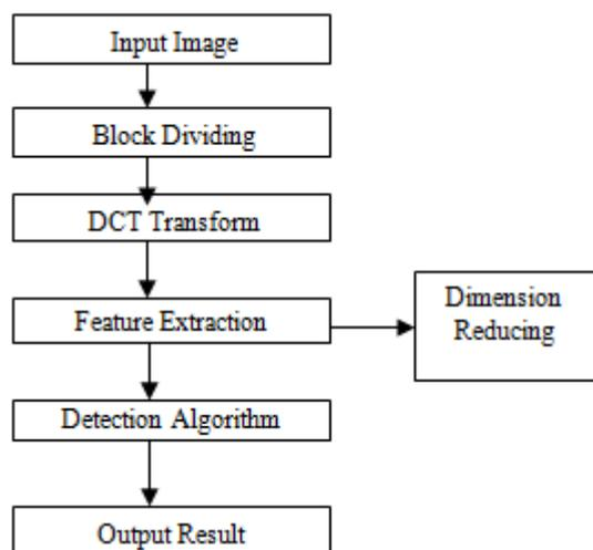
Figure 2: Flowchart of copy-paste forgery detection algorithm
