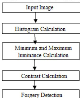
**Figure 1:** flowchart of global contrast enhancement detection algorithm
